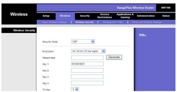
Delete the current key enter the new key. When done click on "Save Settings" on the bottom of the window.
