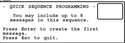
**STEP 4:** Select the desired font for the first message. Three line (normal) will produce the same display appearance as a conventional (non full matrix) 3-line by 8-character message board.
