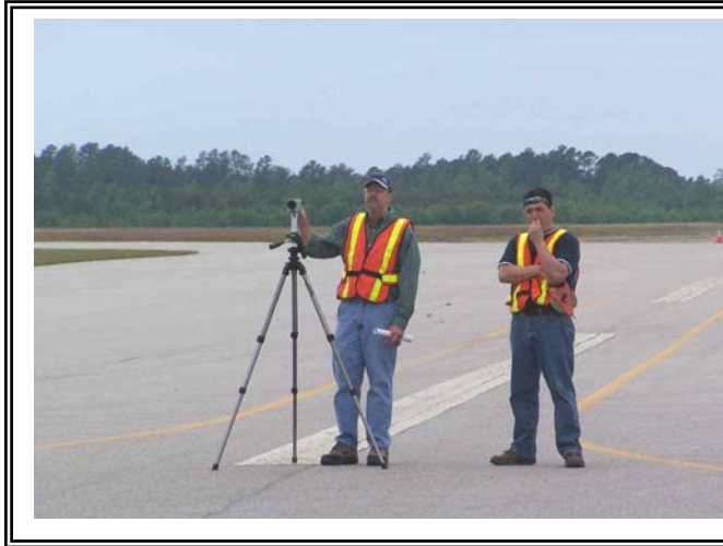
Luminance meter setup
