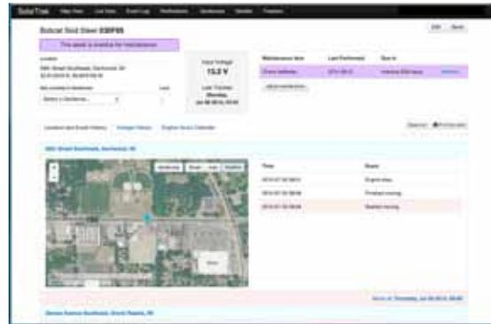
See current location by address and GPS coordinates, by geofence, battery voltage and maintenance reminders from the Details screen. Tabs have Movement History (street or satellite views), Voltage and Engine Hours.
