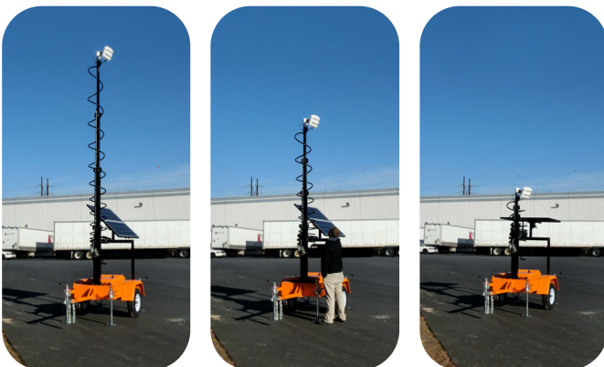
Easy to use hand crank raises and lowers the mast.
