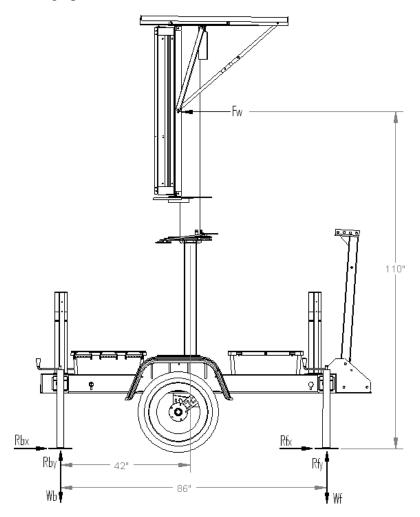
Figure 1: Free body diagram of MBII L&R
