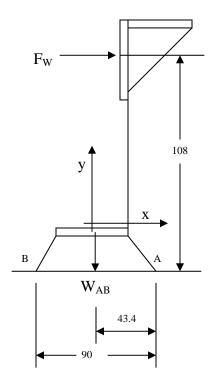
The free body diagram shown above indicates that the center of gravity is located 43.4" from point A. This report will assume that instability of the unit occurs when the unit is in equilibrium with the vertical reaction force  $R_{by}$  equal to zero indicating that the jack stands at point B carry no load. The report will also assume that the wind force acts uniformly on the sign case and therefore can be represented as a single force located at the center of the sign panel.
