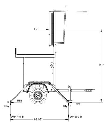
This report will assume that instability of the unit occurs when the unit is in equilibrium with the vertical reaction force at the jack stands is equal to zero indicating that the jack stands carry no load. Since the weight at the rear jack stands  $W_b$  is less than the weight at the front jack stands  $W_f$  the unit will tip over towards the front first. Therefore the instability condition will occur when the reaction force at point  $B\left(R_{by}\right)$  is equal to zero..
